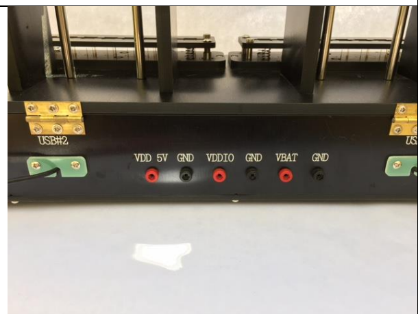
Figure 4 Back View Showing Power and Ground connections
